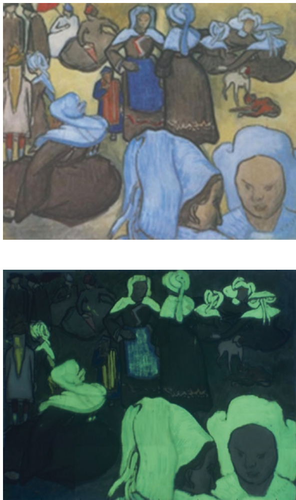
Fig. 8.9 Luminescence from Vincent Van Gogh's painting on paper «Les bretonnes et le pardon de pont Aven», Galleria dell'Arte Moderna, Milano (bottom). Here the bright green emissions from Zinc White (top) are apparent where the white pigment is mixed with blue in the multiple headdresses of the figures in the painting. Other emissions are seen in the yellow paint, and are likely from a Cd-yellow. (Reproduced with permission from Comelli et al. (2012))
