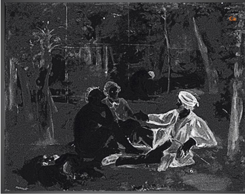
Fig. 15.15 MA-XRF scan for Ca showing grid beneath the Courtauld painting, image from (Amato et al. 2020)
