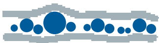
Example of poorly sorted powder with a high proportion of fine particles.
