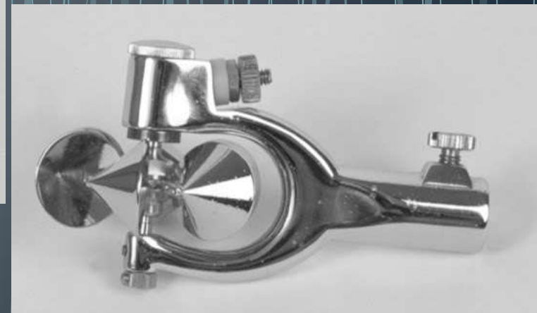
Figure 4-5 Price current meter and 30-lb C-type sounding weight. (U.S. Geological Survey.)
