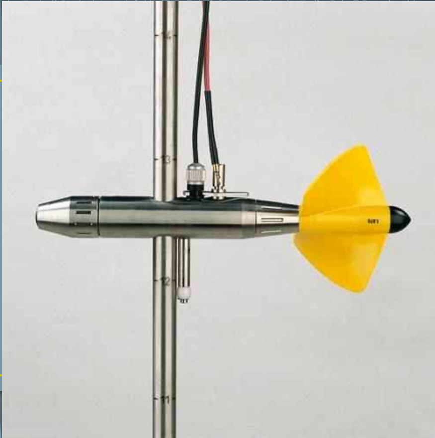
Figure 4-5 Price current meter and 30-lb C-type sounding weight. (U.S. Geological Survey.)
