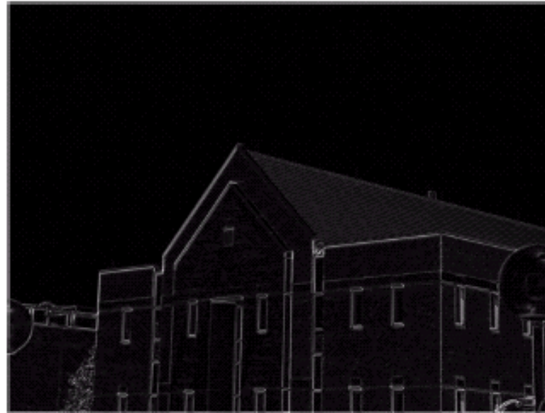
FIGURE 10.12 Diagonal edge detection.
