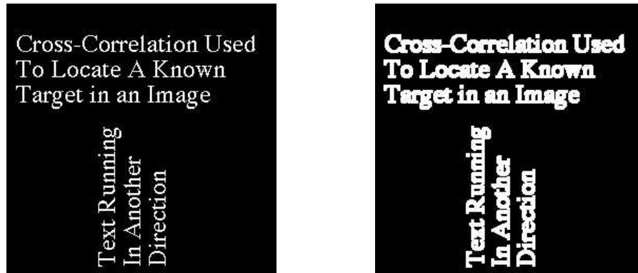
Figure 9.5: Dilation of a binary image
