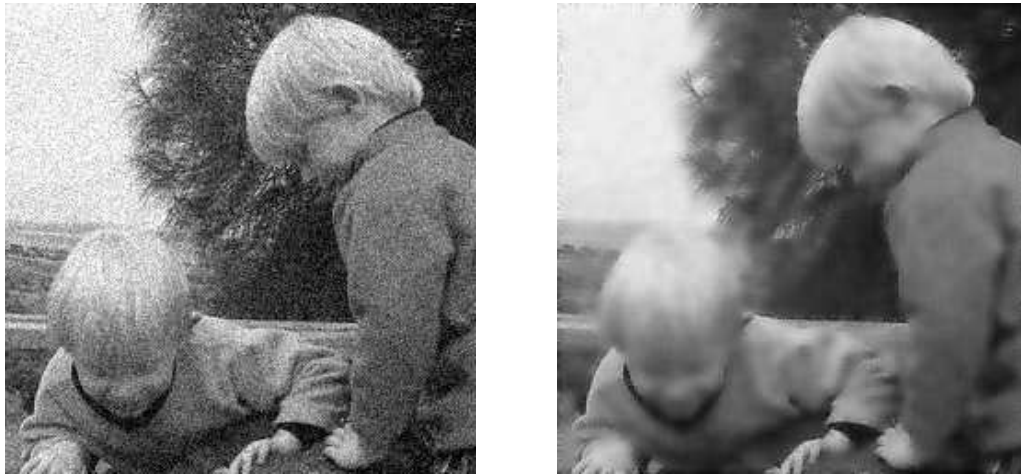
Figure 5.13: Using adaptive filtering to remove Gaussian noise with low variance
