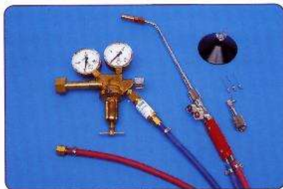
Multiplex melting unit 1 for natural gas/oxygen; check valve, shut-off valve, pressure reducer for oxygen
