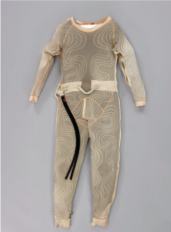
Liquid-cooled suit from the 1950s developed by the Royal Aircraft Establishment, England, and used under aeronautic pressure suits for flying at high altitude. The cooling pipework is woven through the material.
