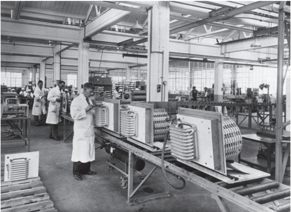
Distinctive Monitor Top compressor units on the assembly line in Britain, c. 1930s.
