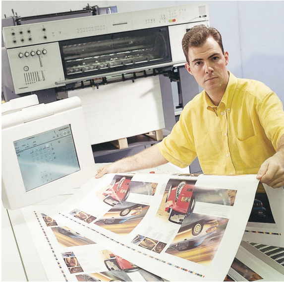
Fig. 2.1-128 Printed sheet taken from the delivery of a sheet-fed offset press for quality control purposes (Heidelberg)
