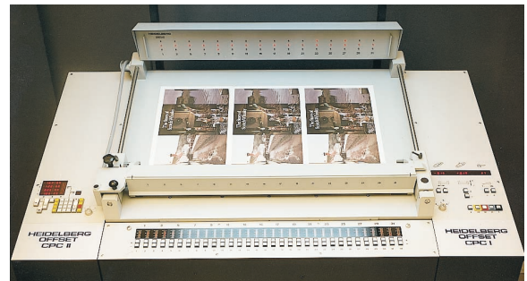
Fig. 2.1-130 Densitometer measuring bar for simultaneous color control patches measurements according to ink zones on the printed sheet on the press control console, with color variation displayed zone-wise (CPC I & CPC II, Heidelberg/Gretag)
