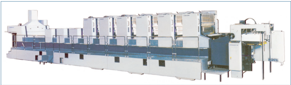
Fig. 2.1-174 Lithrone 40, 6-color press, two coating units, unit for intermediate drying, hot-air extraction in the delivery; sheet size 720 mm × 1030 mm, printing speed 15000 impressions/hour (Komori)
