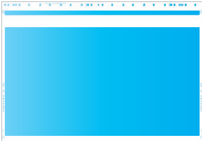
Printed sheet with lateral ink fading for determining the ideal coloration value
