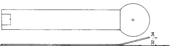
22 Sloping circle without hazards, to be played only from the tee (lane without borderline)
