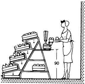
⑧ Counter with stands for boxes and baskets, drip pan and dirt trap
