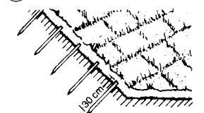
7 Turf on slopes of more than 1:2 fixed with pegs
