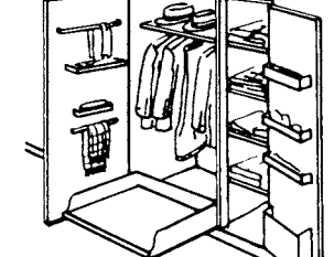
16 Built-in clothes cupboard using the doors for storage
