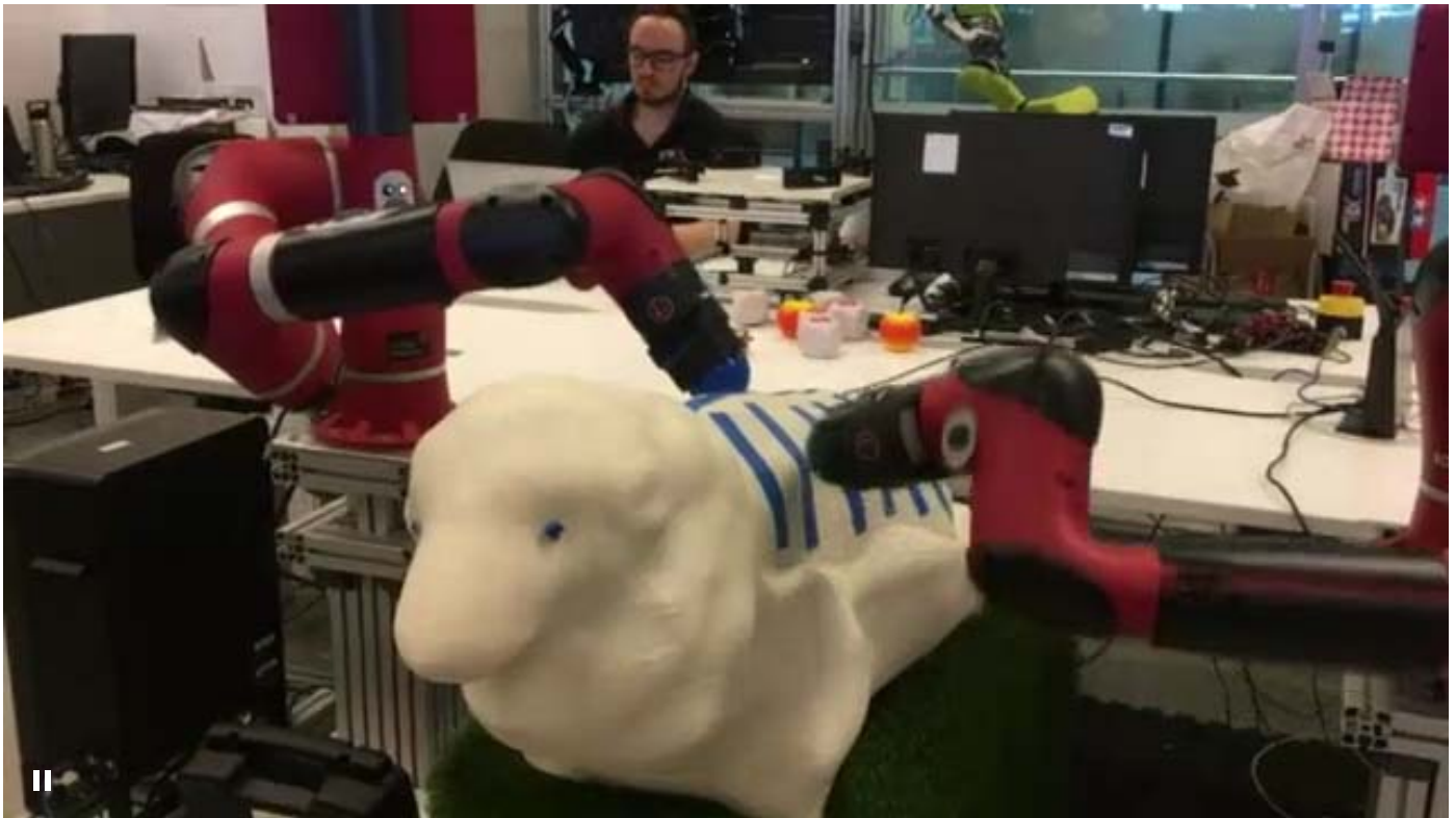
GIF: Robotic arms simulate shearing a 3D-printed sheep
