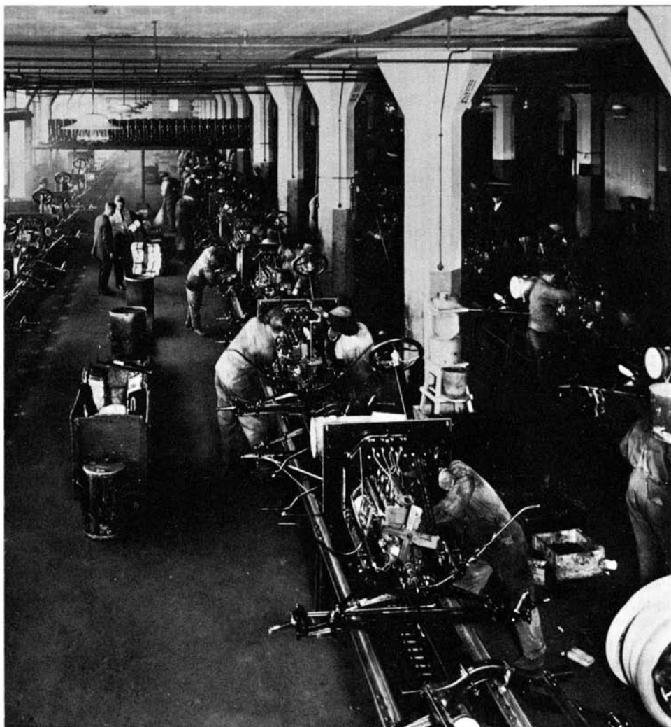
FIGURE 6.32. General View of "The Line," Highland Park, 1914. When Horace Arnold toured the Highland Park factory in 1914 and wrote of the assembly line that assembled a car in ninety-three man-minutes, this is the line of which he was speaking. (Henry Ford Museum, The Edison Institute. Neg. No. 833-987.)
