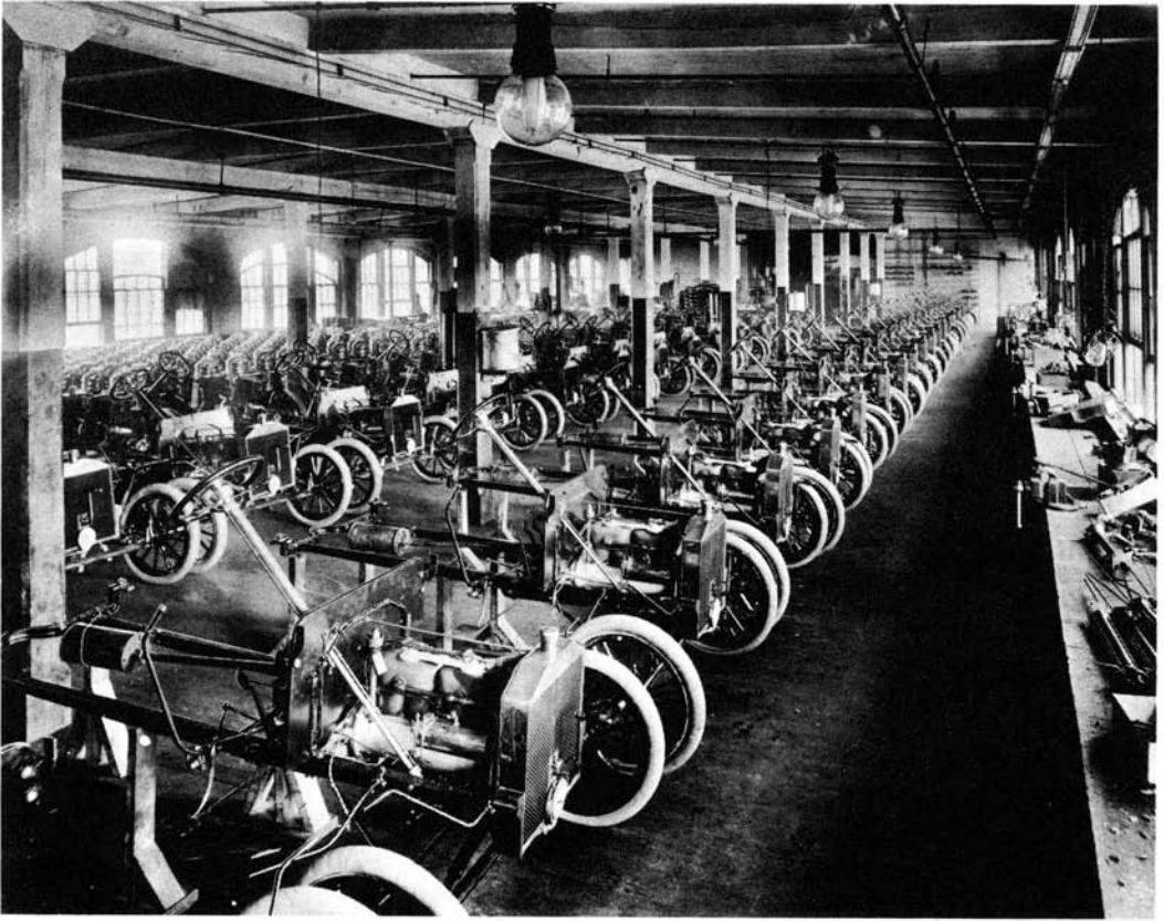
FIGURE 6.2. Static Assembly, Model N, Ford Motor Company Piquette Avenue Factory, 1906. The cramped condition of the Piquette Avenue factory would soon lead Henry Ford to expand the plant in 1907 and build the Highland Park plant, which opened in 1910. (Henry Ford Museum, The Edison Institute. Neg. No. 833-37306.)
