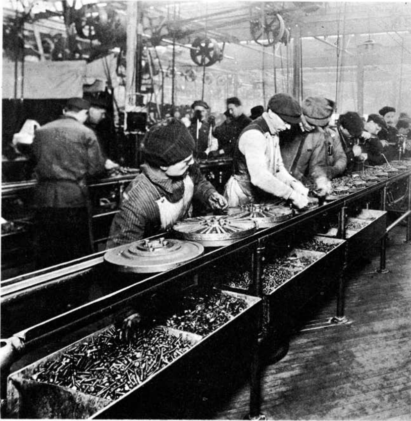
FIGURE 6.23. "The First Magneto Assembly Line," 1913. This is a photograph of what Allan Nevins, among many other historians, called the first magneto assembly line. In his text, Nevins said that the magneto coil assembly was the first subassembly to be put on a line basis, but this illustration shows assembly of the flywheel magneto, the other half of the entire Model T magneto. (Henry Ford Museum, The Edison Institute. Neg. No. 833-167.)
