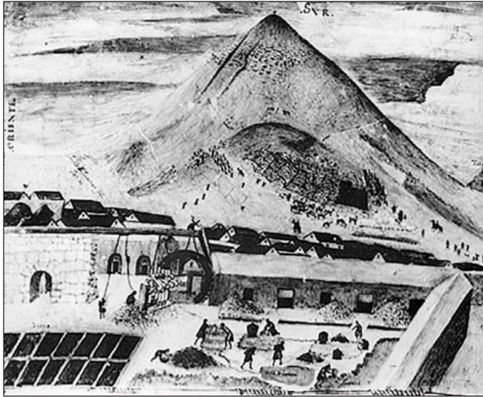
FIG. 1 The Cerro Rico of Potosí. The foreground illustrates the patio amalgamation process, the technological development in silver refining that arrived to the area with Viceroy Toledo in the early 1570s. (Source: Courtesy of the Hispanic Society of America, New York, Ms. K3.)
