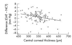
Figure 1 Differences between intraocular pressure measurements made with the Goldmann applanation tonometer by observer 1 and those made with the Canon TX-10 non-contact tonometer plotted against central corneal thickness.
